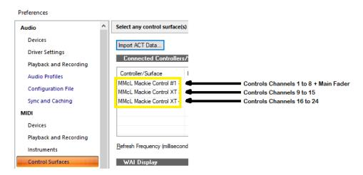
The fader offset assignment is made at the time you add your controllers within Cakewalk's Control Surfaces preferences, so you can override the automatic fader offset assignment by using the "Configure Layout" button.
