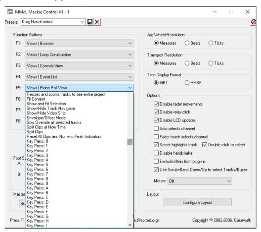
When used in conjunction with the Key Bindings within Cakewalk, this can greatly enhance the functionality of the function buttons over the standard list of commands, e.g. by configuring an MCU function button to run a CAL script.
